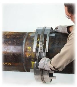
**PSR-2000-XX** Piper Steel Rail Easily Installed on the workpiece for quick installation and removal
