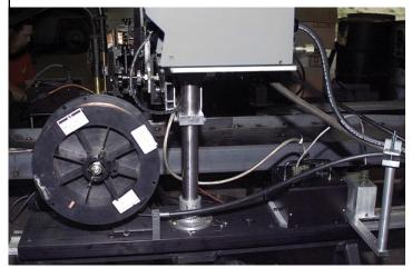
BUG-2785 Carriage 36" (914 mm) mounted on Bug-O ARR Rail Used as part of a Dual Torch Beam Welding Gantry
