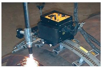
Hi-Flex Rail (FMD) for various circumferential and irregular surface applications down to 30" (760 mm) radius (Page 2)
