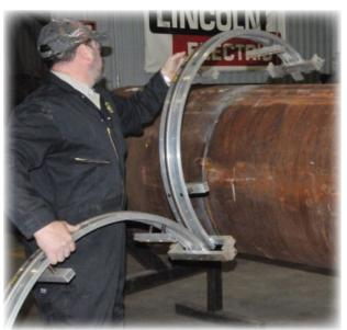
**BRR-3250-XX** Bent Rigid Rail Easily Installed on the workpiece for quick installation and removal
