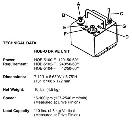
**\*NOTE:** Speed and load ratings apply at radius of ring gear. Speed is proportional to radius at any other point, and load rating is inversely proportional to radius.
