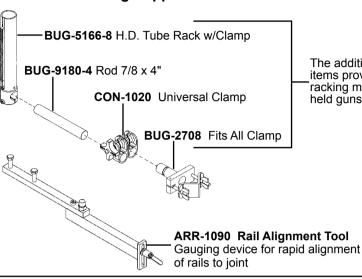
The addition of these 4 items provides a vertical racking motion for hand held guns.
